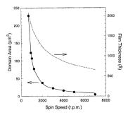
Fig. 4. Average domain area and film thickness as a function of the spin speed during spin coating.
