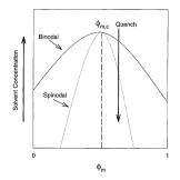
Fig. 1. Schematic ternary phase diagram of a two polymer/solvent system.
