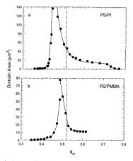
Fig. 3. Average domain area versus PS mass fraction for (a) PS/PI blend films and (b) PS/PIMAA blend films on Si-SiO<sub>x</sub>. The curves are intended to guide the eye. The vertical dashed lines correspond to  $\phi_m = \phi_m c$ .
